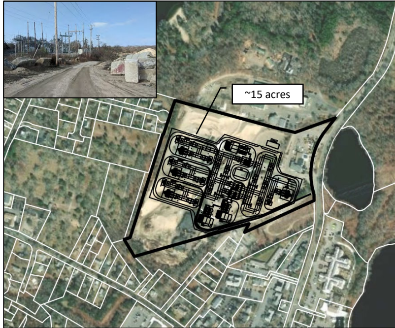
HVAC Substation Layout at Preferred Site
